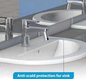
It is **MANDATORY** that the system should feature anti-scald protection at every draw off point to protect users in the event of accidental use during the thermal disinfection cycles. The cartridges will cut off the water flow whenever the temperature exceeds 48 °C.
